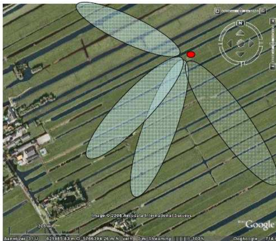
Fig. 2. The projection of the footprints of the EC masts clockwise, averaged over: 16 March, Aug-Nov 2006, 12 July and 8 Nov estimated by the model of Kormann and Meixner (Kormann and Meixner, 2001; Neftel et al., 2007).
